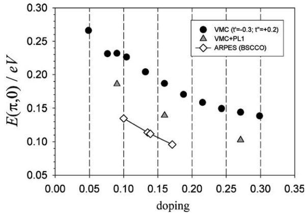
Fig. 3. Comparison of the excitation energy at  $(\pi/0)$  calculated using the RVB WF, that after first order Lanczos method (VMC+PL1) and the experiments (see text). Note that the optimal doping determined by the RVB WF is around 0.30 and decreases as the WF is improved by PL1.
